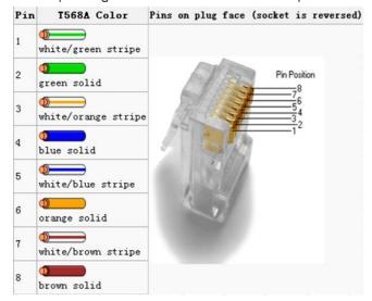
3. Guide the cable gland and communication panel over the network cable and then connect the RJ45 plug to the RJ45 keystone socket.
