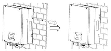
If a second protective conductor is required in your country, ground the inverter and secure it so that it cannot be lifted off the wall bracket (see section 5.4.3 "Second protective grounding connection").
