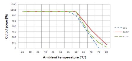
Power reduction with increased ambient temperature (TL1000-20) Output Power[W] -150V 360V -450V Ambient temperature [C]
