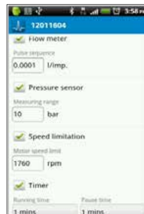
Fig. 8b: Pump system settings 2
